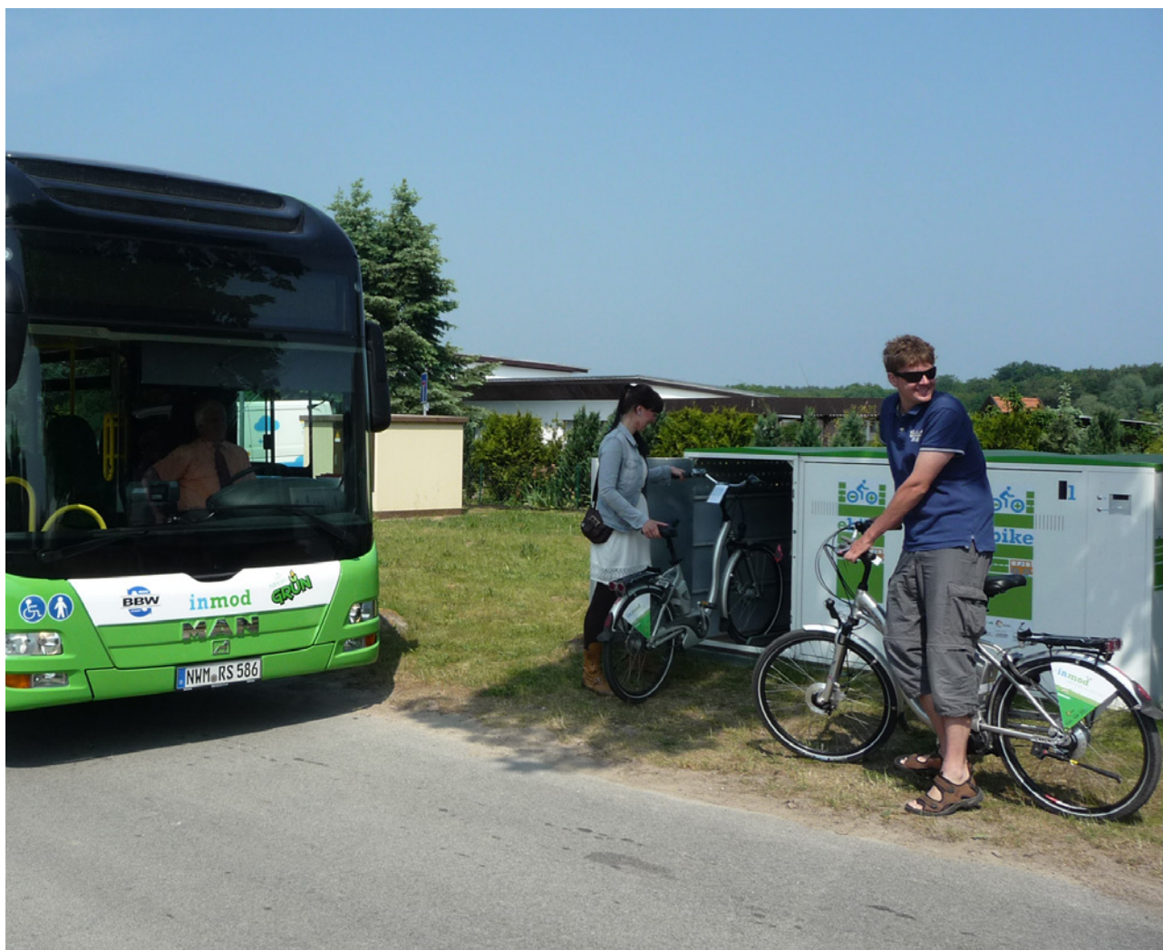
Pilotproject "INMOD – elektromobil auf dem Land" (INMOD – Electromobility in rural areas) in Mecklenburg-Vorpommern: hybrid bus with pedelec connection. Hire pedelecs are available from secure bike lockers with integrated charging stations.
